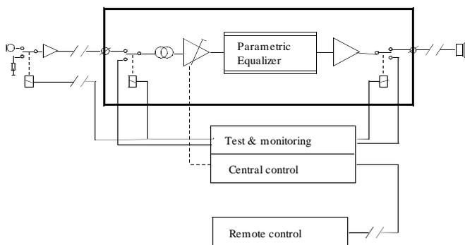
FIGURE 3. A typical amplification channel of a MCR system.
