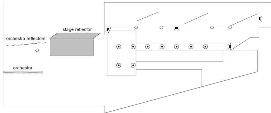
**Figure 9:** Microphone and loudspeaker positions.
