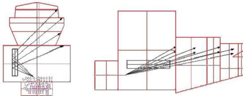
**Figure 3:** First order reflections with straight oriented specular right angle reflector.
