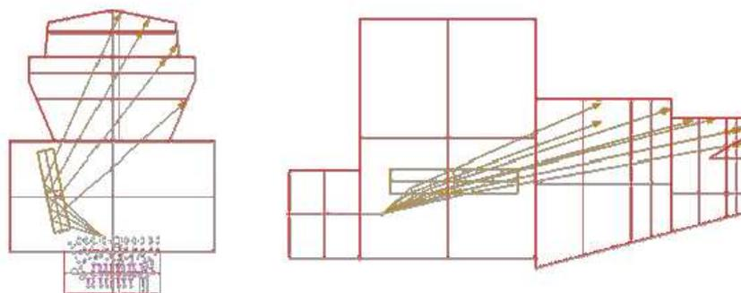
**Figure 4:** First order reflections with angled (in plan) specular right angle reflector.
